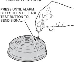
A TEST SIGNAL WILL BE SENT A FEW SECONDS AFTER THE SWITCH IS RELEASED
