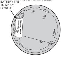
3-VOLT LITHIUM BATTERY - TYPES: DURACELL DL123A, PANASONIC CR123A, SANYO CR123A, ADEMCO 466. AVAILABLE AT LOCAL RETAILERS AND INTERNET SUPPLIERS. **NOTE**: USE <u>ONLY</u> THESE SPECIFIC BATTERY MODELS.
