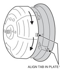
ALIGN TAB IN PLATE WITH NOTCH IN COVER
